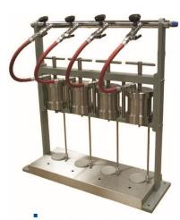
The Filter Press assemblies consist of a reservoir mounted in a frame, a pressure source, a filtering medium and a graduated cylinder for receiving and measuring filtrate.
