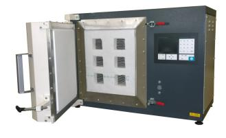
In this style of kiln a fixed gradient of approximately 20/25°C would be apparent between each of the nine measuring point. Overall there is an approximate gradient of 180°C across the nine thermocouples between the "hot" and "cold" ends.
