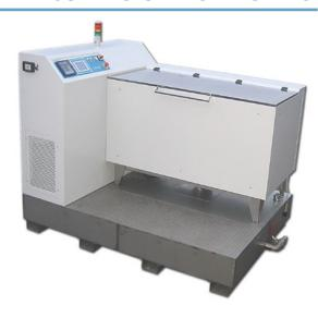
Tank for determining resistance to frost, model DFR/60
