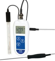
The 8100 pH and temperature meter features an easy to read, LCD display and is supplied as a kit which includes a 8100 pH meter, general purpose combination glass electrode, temperature probe, 4.01 and 7.00 pH buffer solutions and carrying case.
