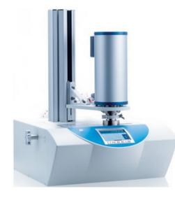
**DTA** uses a dynamic measuring principle. This instrument will measure endothermal and exothermal heat flow between the sample and reference (enthalpy).
