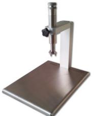
Instrument for determining the apparent density (porosity) of raw ceramic tiles
