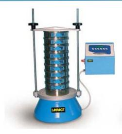
**SV001** motorised bench mountable shaker, suitable for sieves up to 315mm. The sieving action is provided by an off set weight motor which imparts random multi-directional motion to the sieve stack. The action provides and ideal movement for particle sizes up to 20mm. A timer is fitted to provide automatic stop on completion of test.
