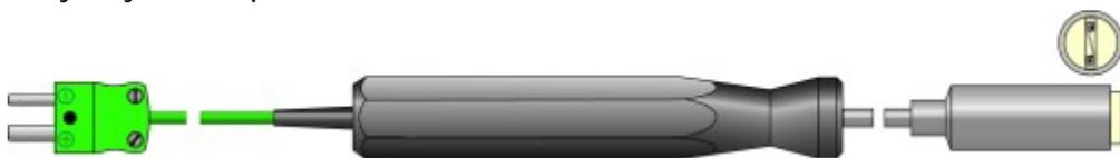
These heavy duty, high temperature, surface probes are ideal for measuring the temperature of griddles etc. A right-angled version is available. Dimensions  $\text{Ø}12 \times 130$ mm, Maximum tip temperature  $+1000^{\circ}\text{C}$ .
