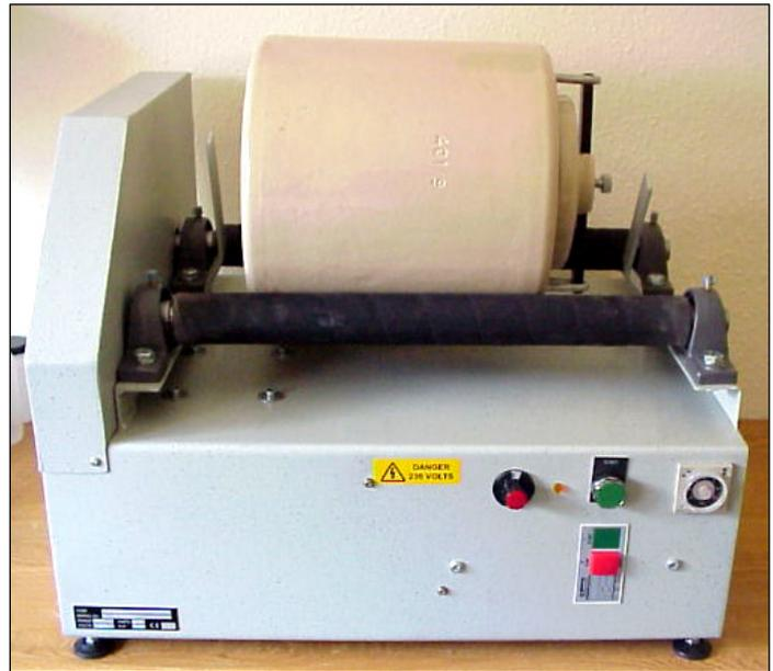
G90 Jar Mill with optional timer and variable speed motor.
