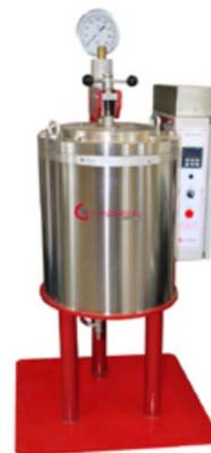
“Crazing” is formed by small cracks appearing in the glazed surface of the test piece. The resistance to crazing is determined by subjecting the test piece to high pressure steam in the tank. Once the cycle is complete a coloured dye is washed over the glazed surface and wiped off. If crazing has occurred, the dye will enter the cracks and will remain after the excess is wiped off.
